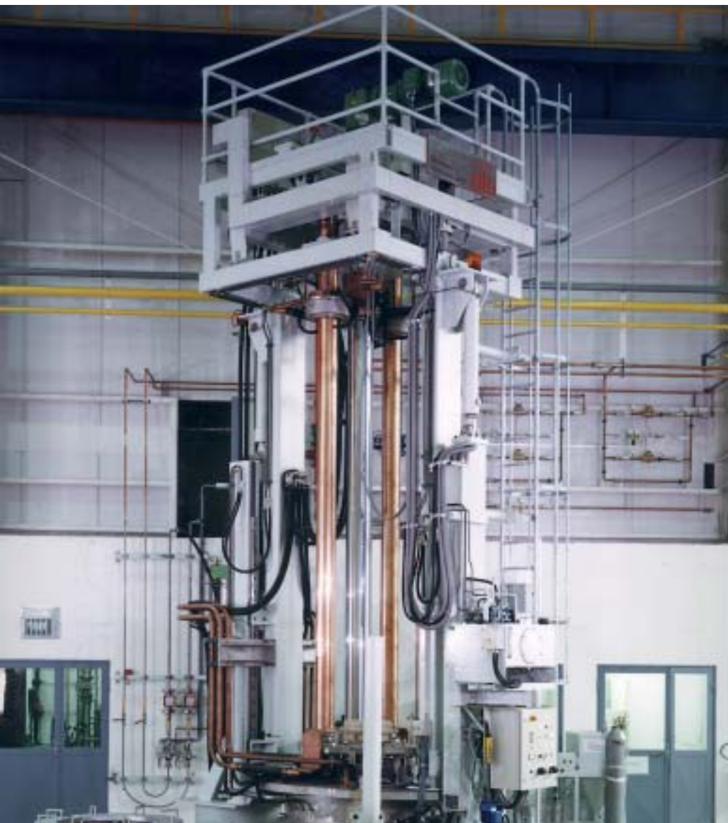
16 ton PESR furnace, max. 16 bar.
