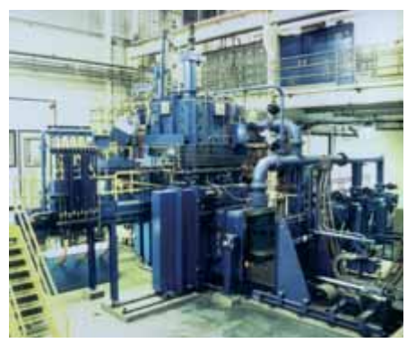
Horizontal Furnace VIM-IC 40 E/DS/SC for the Production of large E, DS and SC Components
