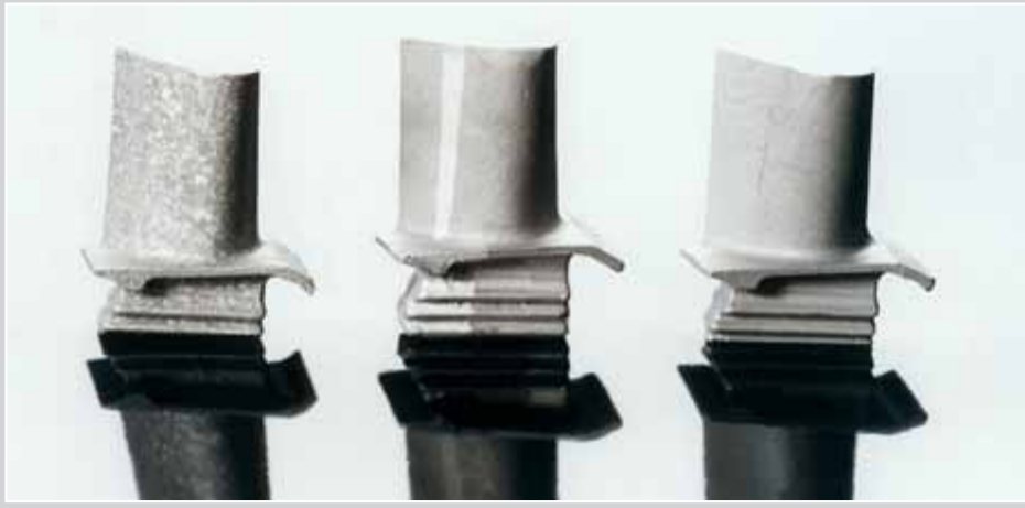
Turbine Blades with Equiaxed (E), Directionally Solidified (DS) or Single Crystal (SC) Structures
