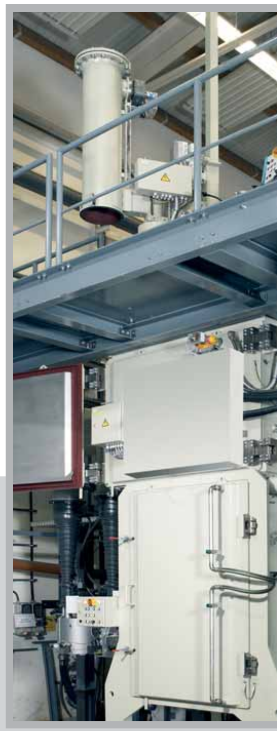
VIM-IC 10 E/DS/SC with Double Door Design for quick Change from E to DS/SC Operation and Vice Versa.
