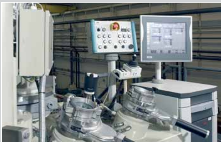
Main Control Station - Visualization Monitor with Touchscreen
