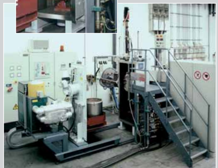
VIM-IC 0.5 DS/SC/LMC R & D Furnace for the LMC Process
